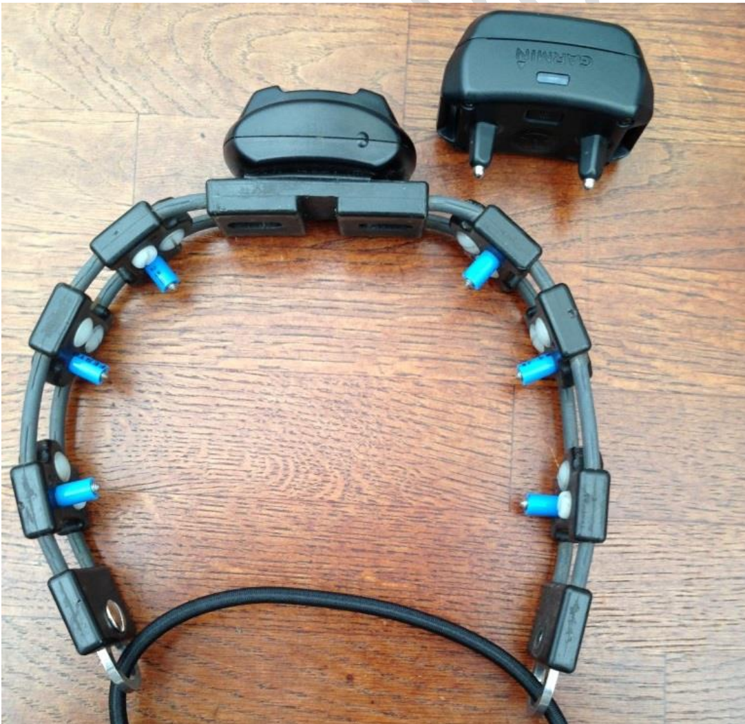
Chameleon® Extenders long (triple contact) with normal contact points and linked with micro collar (MS) and Garmin:
